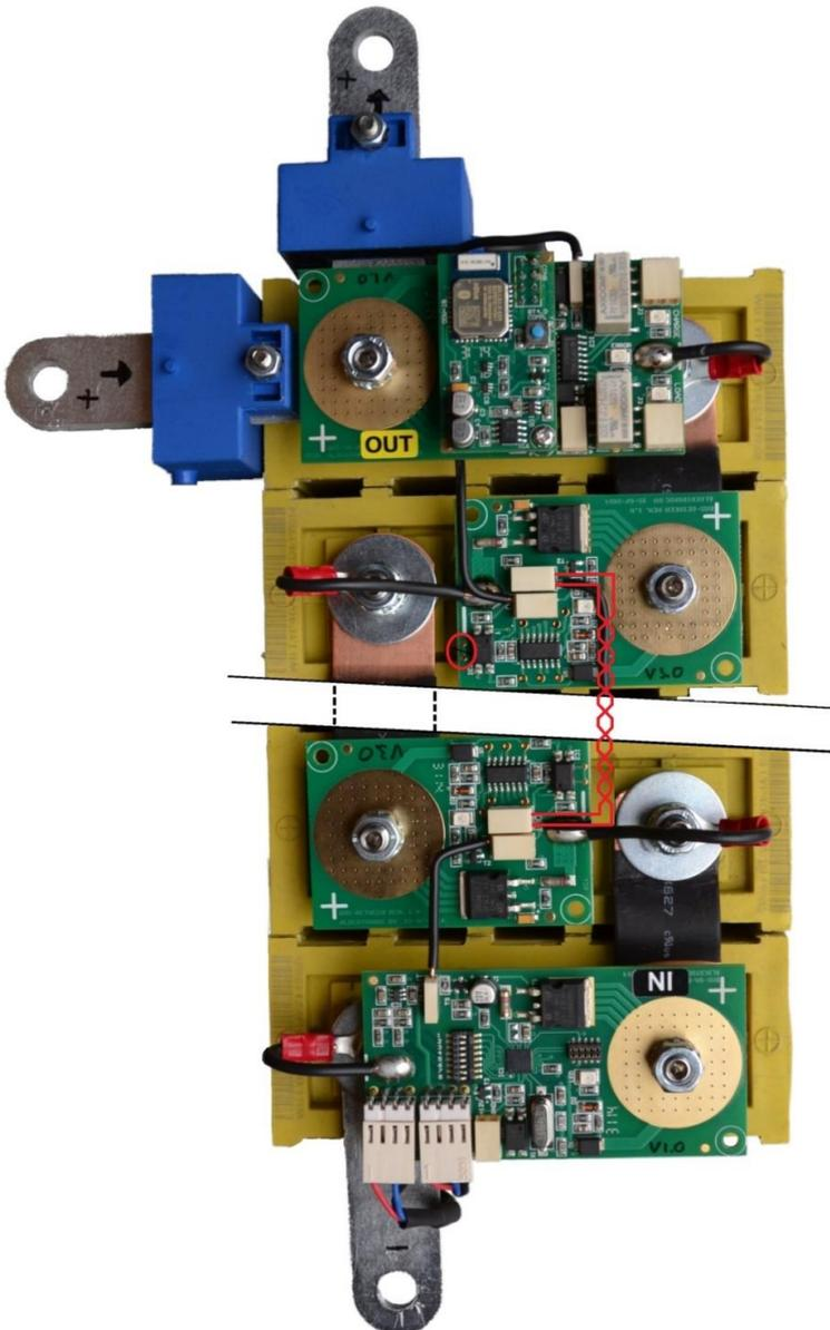
When the battery pack has separated battery banks the interconnection has to be changed to prevent interference from other components in the system. The data connection has to be galvanic isolated. This can be done by the following procedure:
